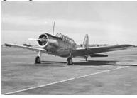
It had a two-seat tandem cockpit with a full set of flight controls for student and
