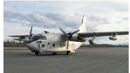
The Provider could carry 60 troops or 50 stretchers. Some had a pair of under-wing mounted turbojet engines that increased payload, shortened its takeoff distance, improved climb rate and added safety in the event of a radial engine failure. It had a crew of 3 or 4 depended on mission, cruise was about 150kts, range about 900nm and MTOW 60,000lbs.
